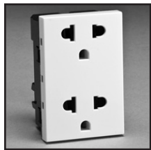
85100X45D Brazil NEMA 5-15R & CEE 7-16 Duplex Outlet 16A-250V & 15A-127V 67.5x45mm
