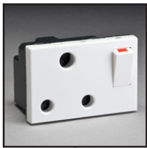
73100X45 S. Africa, India and UK BS 546, SABS 164-1 & IA 16A3 Switched Outlet 16 Amp 250V 67.5x45mm
