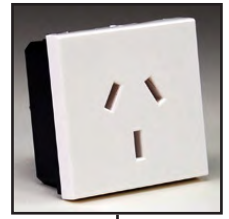
84100X45 Argentina IRAM 1073 Outlet 10 Amp 250V 45x45mm
