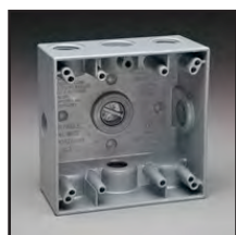
79430 Surface Mount Standard American 4x4 Wall Box. Cast Aluminum. 1/2 inch NPT Entries. Use with 4x4 Mounting Frames and Wall Plates.
