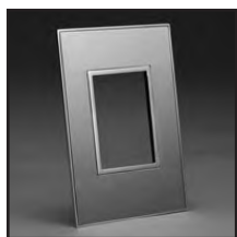
79185X45-N Finish Plate. Brushed Stainless Steel. Fits 79170X45-N Mounting Frame. Opening Size 67.5x45mm.
